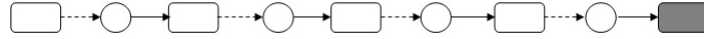
Figure 3.5 Chain of hold-and-wait dependencies while trying to acquire a lock leading to a deadlock.
